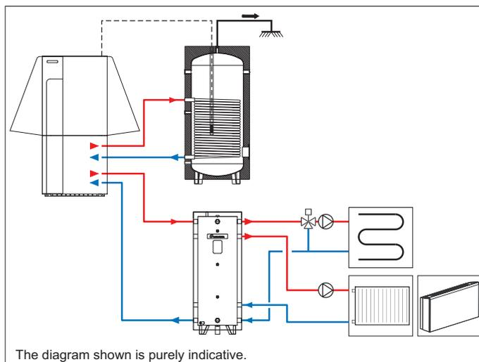
The diagram illustrates the use of the BT/TP storage tank as a storage tank on the heat pump return pipe so as to increase the volume of water available in the system, avoiding excessive starts and stops. In this case, make sure the available pressure head of the pump on the unit is sufficient to guarantee correct system operation.
