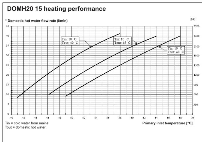
**In this case, a thermostatic valve should be used at the instant domestic hot water production kit outlet to avoid excessive domestic hot water temperatures.**
