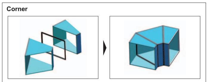
The kit comes with one straight section, 1200 mm long, and a corner piece. These can be used separately to achieve the configuration shown in the figure, thus guaranteeing the specified clearances.
