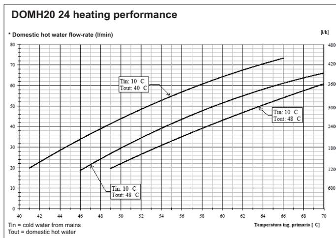
\* The domestic hot water flow-rate shown on the performance curves remains constant for a variable time, depending on the volume of the storage tank. Also see the instructions in the "Selection guide".
